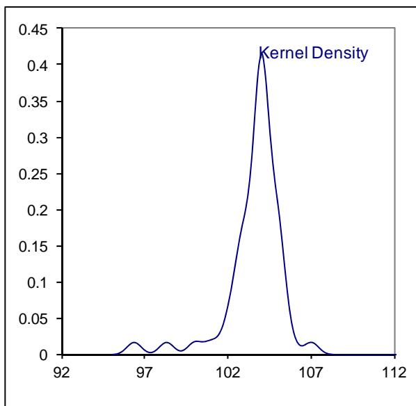
Determination of Kinematic Viscosity @ 40°C (Houillon) on sample #13063; results in mm<sup>2</sup>/s
