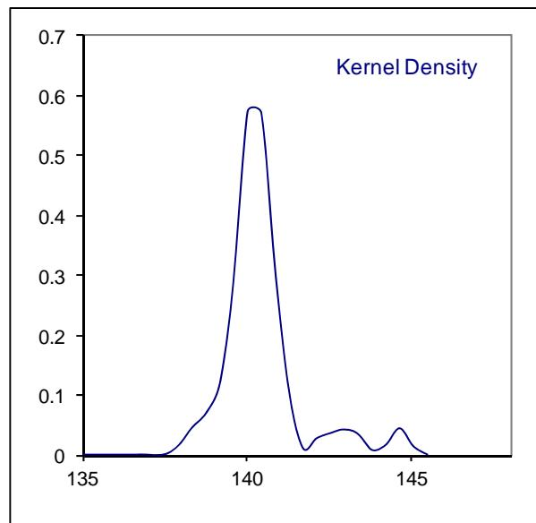
Determination of Kinematic Viscosity @ 100°C on sample #13063; results in mm<sup>2</sup>/s
